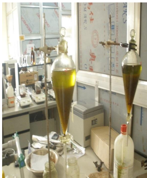
Fig. 2. Fractionation of Moringa oleifera leaf at Faculty of Pharmaceutical Sciences of Nnamdi Azikiwe University, Awka
