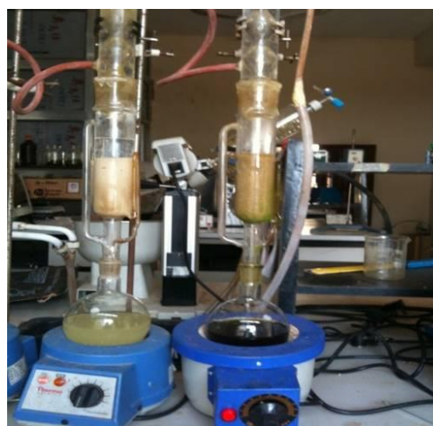
Fig. 1. Moringa oleifera extraction process using Soxhlet extractor at Faculty of Pharmaceutical Sciences of Nnamdi Azikiwe University, Awka
