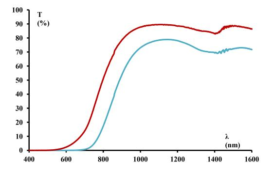
Fig. 3. Evolution of the spectral transmittance of 2 samples. Theme asurement is made with a 1 mm cell at a concentration of 0.1% [10]
