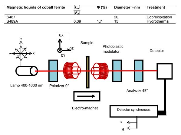
Fig. 1. Installation using the spectral polarimetric photo elastic modulator
