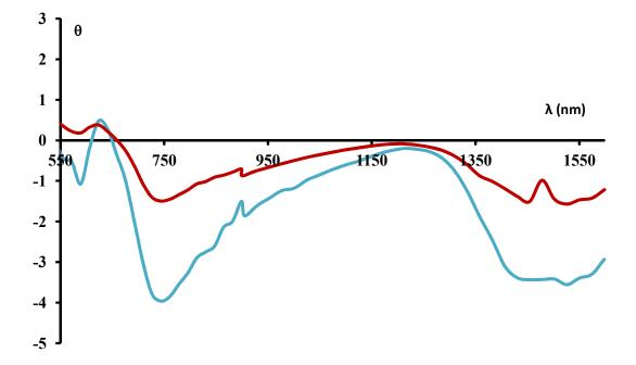
Fig. 2. Spectral evolution of the Faraday rotation saturation of 2 samples. Theme asurement is made with a 1 mm cell at a concentration of 0.1%
