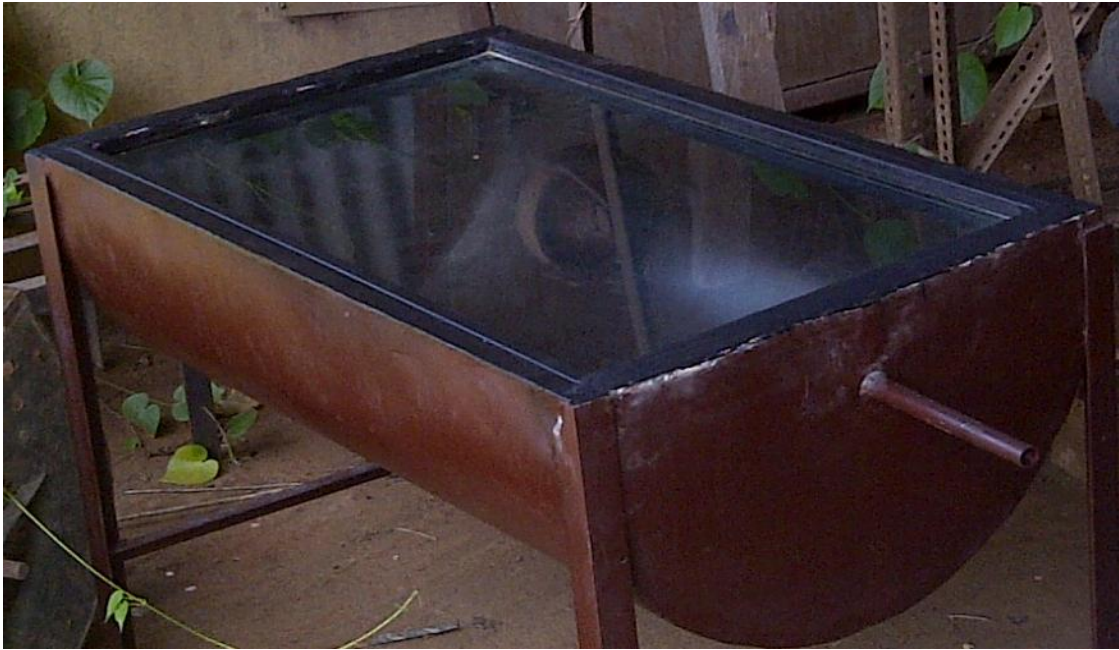
Fig. 3. Heat storage chamber
