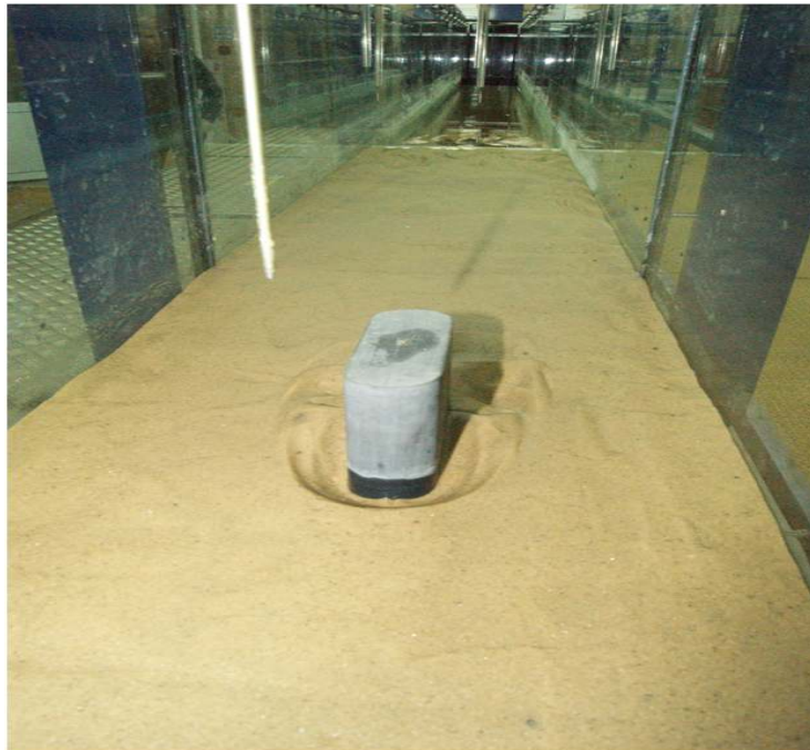
Fig. 2. Round nosed pier picture after the flume dried
