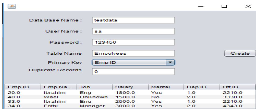
Figure. 9: The analysis quality of a spreadsheet input. The figure shows that there is a duplicate in the "Emp ID" column and PK error in that field, also missing in "Job" column as shown in figure. 2
