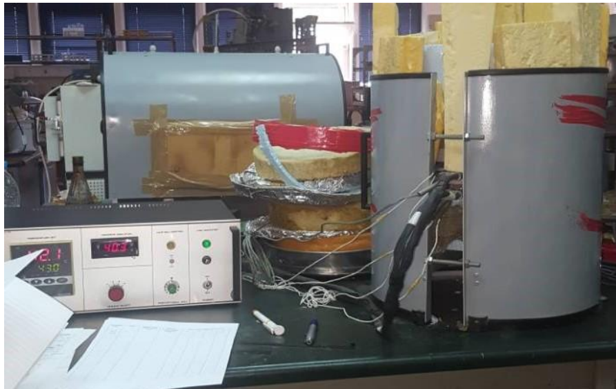
Fig. 4. Thermal conductivity measuring equipment
