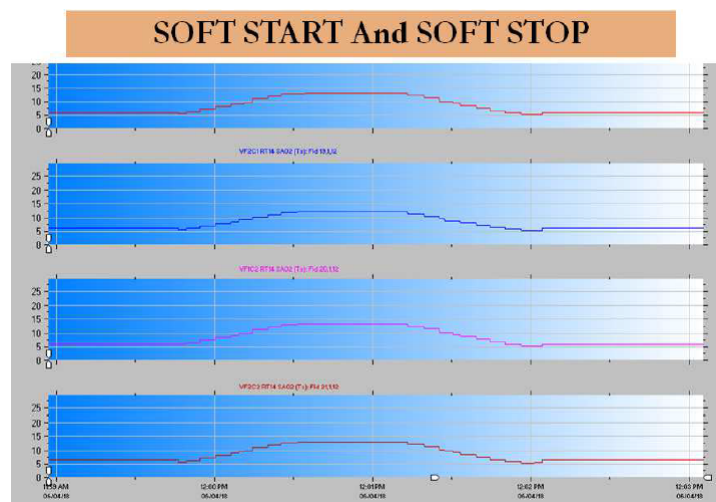
Figure 5. Soft start and soft stop with PWM Enable and disable
