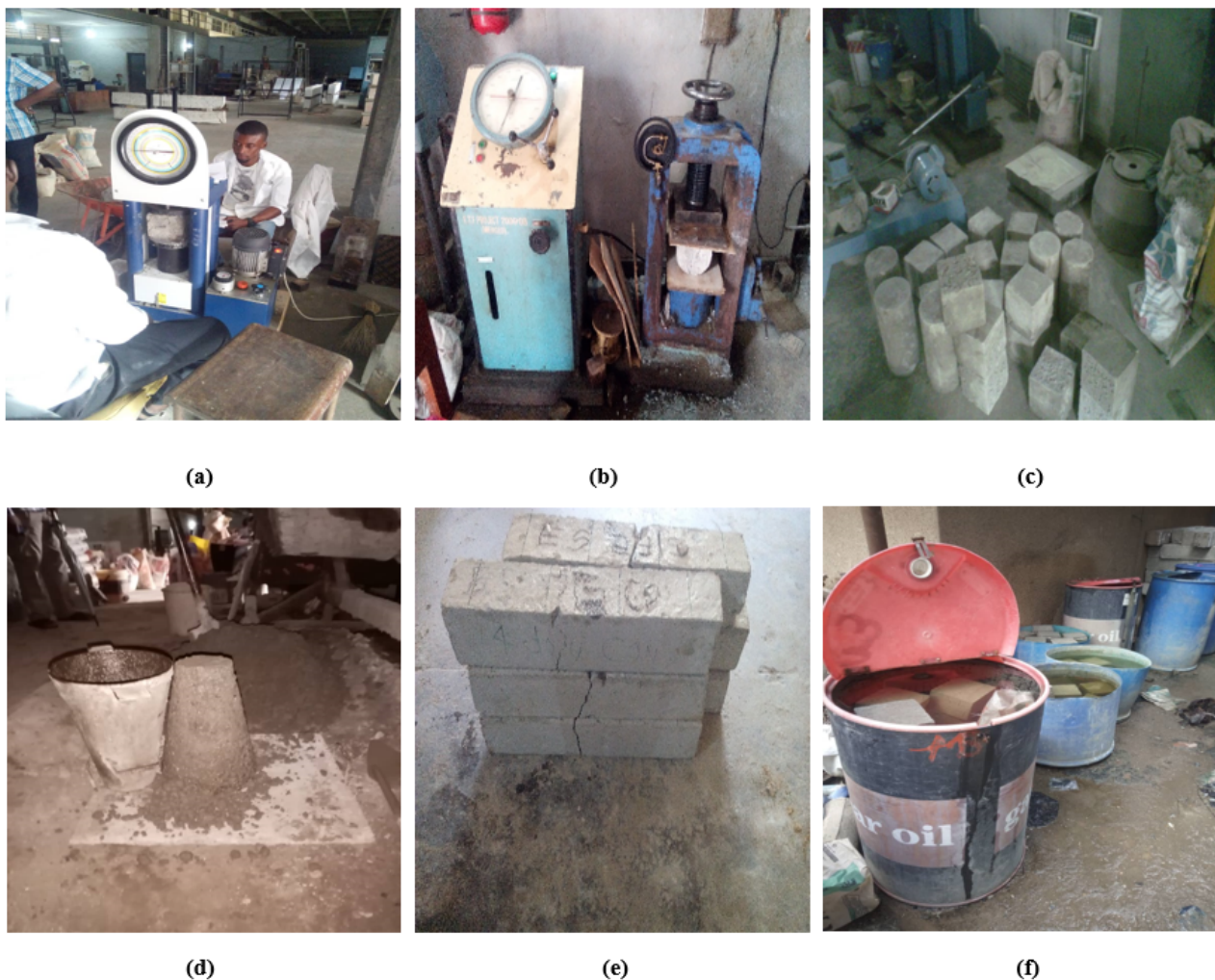
Figure 1. Laboratory Equipment and Experimental Activities (a) & (b) Avery Denson Universal Testing Machine for Compressive and Split Tensile Strength (c) Sample Measurement using Weighing Machine (d) Slump Test (e) Tested Concrete Beams (f) Concrete Cubes Immersed in Curing Media
