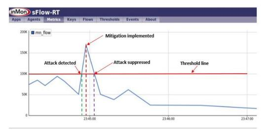
Fig. 7. Phase 3 attack detection and mitigation
