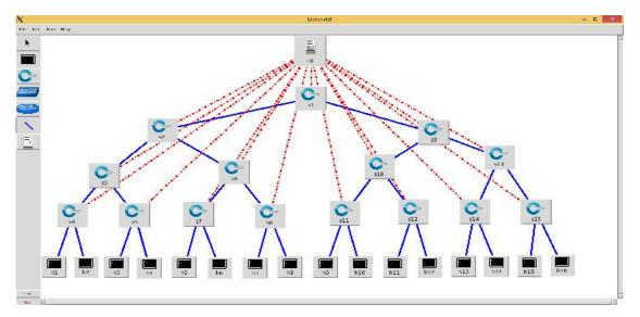
Fig. 4. IPv6 network topology testbed
