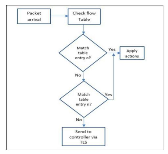
Fig. 1. Open flow packet flow algorithm
