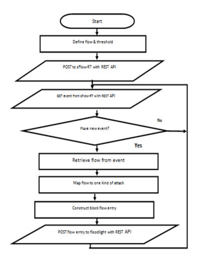
Fig. 3. Mitigation algorithm of IPv6 SDN
