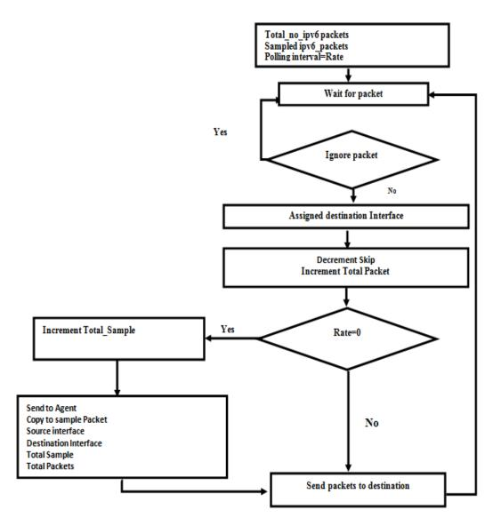
Fig. 2. Data sampling algorithm for IPv6
