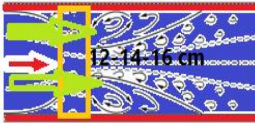
Fig. 2. Flow through a bridge opening
