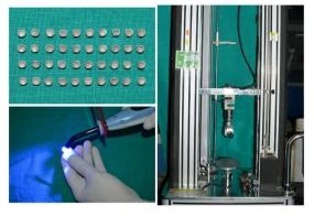
Fig. 2. Recycled brackets, Bonding of the brackets and Universal Testing Machine
