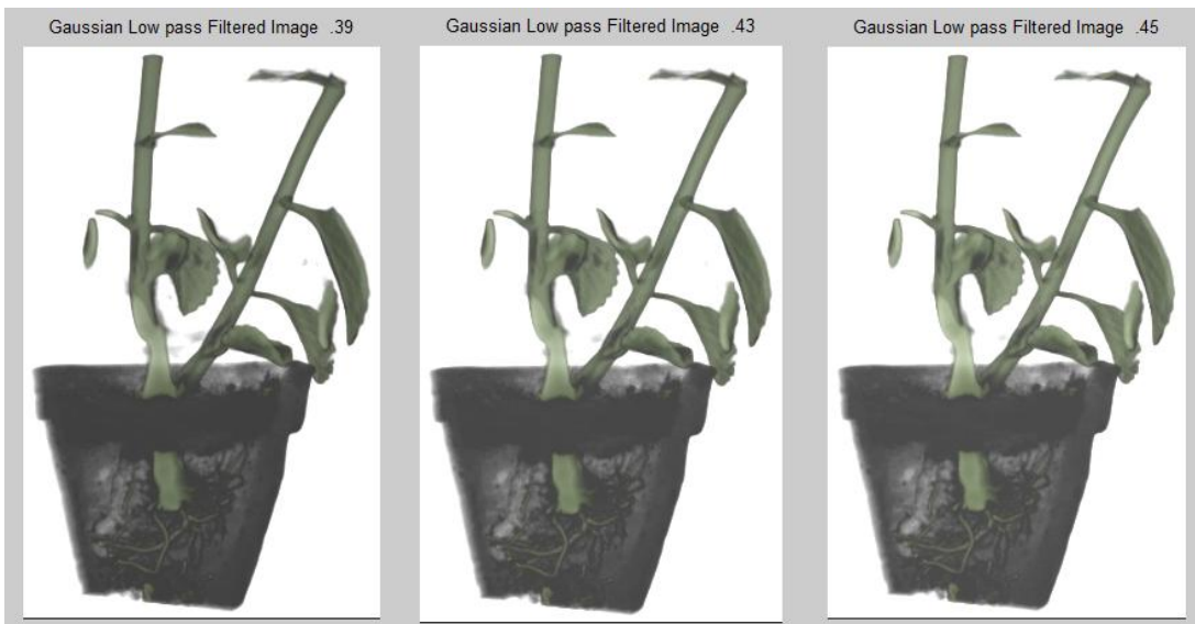
Fig. 5. Processed image by Gaussian low-pass filter with different f_c values
