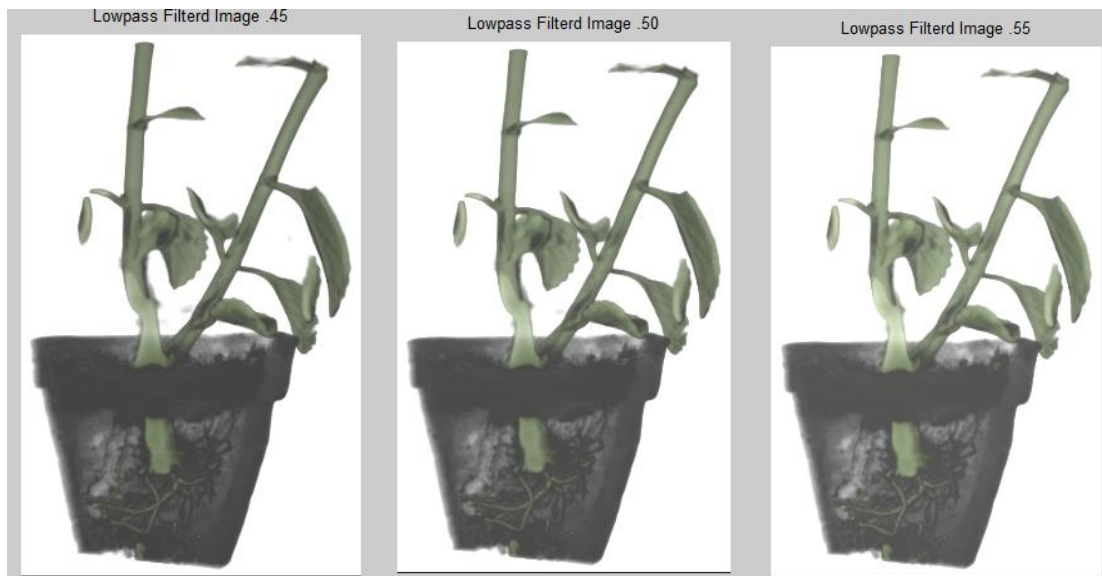
Fig. 7. Processed image by low-pass filter with different cut-off frequencies. The suppression of the noise is pronounced with f_c= 0.50
