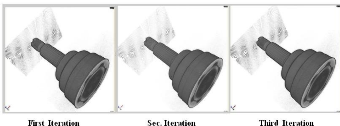
Fig. 13. Noise suppression by the iteration technique
