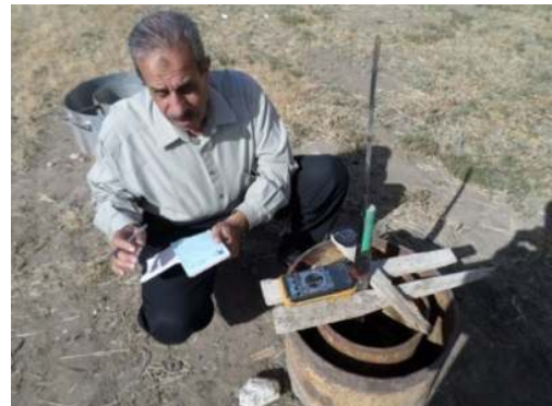
Fig. 2. Utilizing electronic sensor to note the time the water begins to infiltrate into the soil
