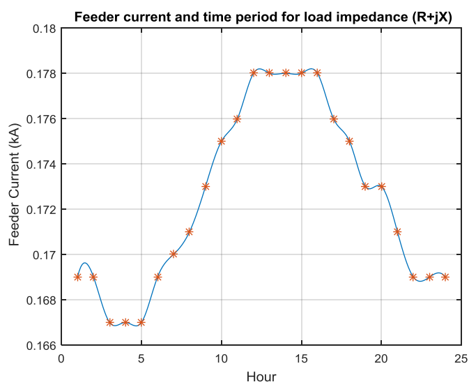
Fig. 7. Feeder current and time period for load impedance (R+jX)
